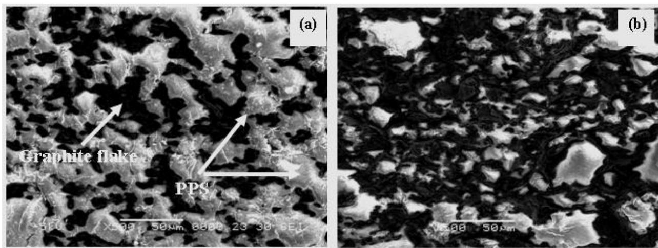
**Fig. 2.** SEM of fractured surfaces of (a) 8 wt% and (b) 20 wt% GF filled PPS composites.
