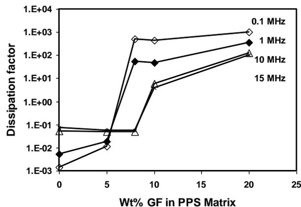
Fig. 5. Dissipation factor for composites as a function of GF content in the matrix.
