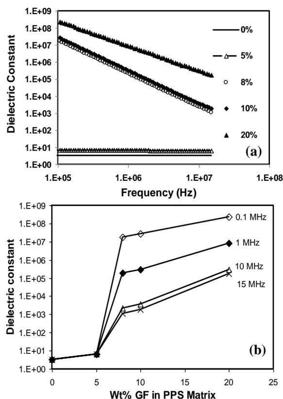
Fig. 4. Dielectric constants for composites as a function of (a) frequency and (b) GF content in the matrix.
