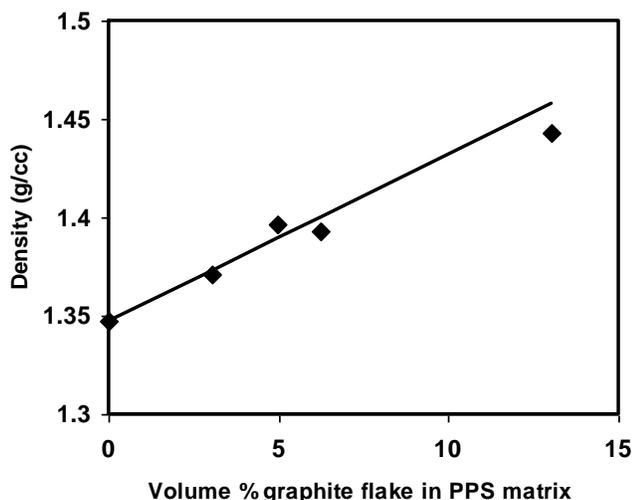
**Fig. 1.** Theoretical and experimental density for PPS/GF composites. Solid line represents theoretical density predicted from a rule of mixture and filled diamonds are experimental data.
