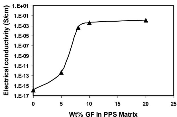
Fig. 3. Electrical conductivity of PPS/GF composites.
